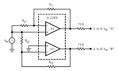
$V_{CC} = V_{CC} = 5V$   $R_{f1} = R_{g1} = 590\Omega$ , 1%  $R_{f2} = R_{g2} = 610\Omega$ , 1%
